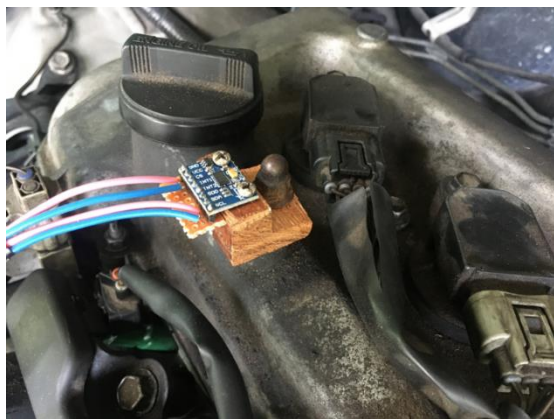
Fig 2: Accelerometer fixed rigidly to the engine block.
