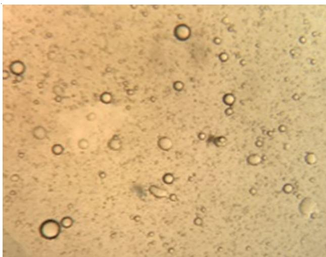
Fig. 1. Microscopic image of the LGO-CS-MCs formed at 3 g of LGO, 1% of CS and 0.5 g of STPP
