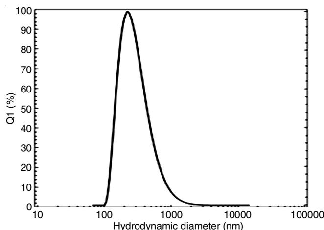
Fig. 3. Particle size distribution of dried LGO-CS-MC
