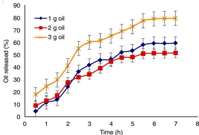
Fig. 6. Effect of variation of oil loading on release profile
