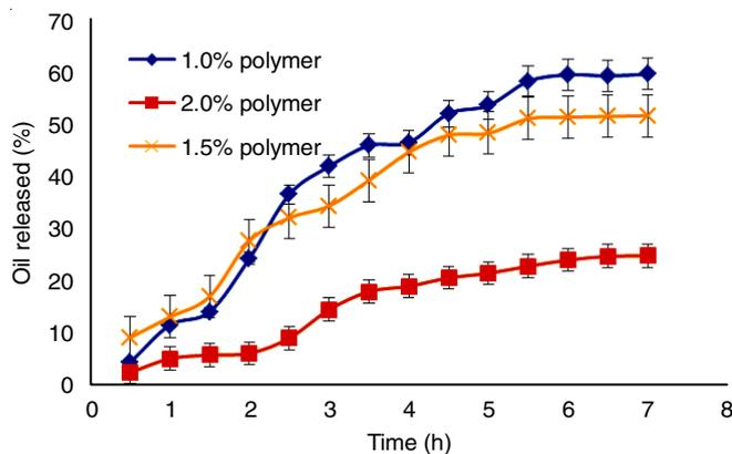
Fig. 7. Effect of variation of CS concentration on release profile
