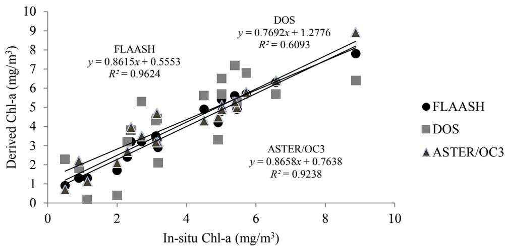
**Figure 3: Comparison between estimated Chl-a using the DOS, FLAASH and ASTER/OC3 based methods with in-situ Chl-a.**
