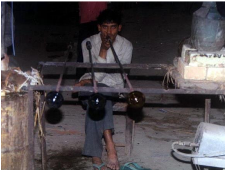
Fig.15. Maintaining the bulb - North India
