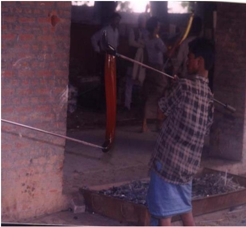
Fig.18 Cooling of the glass mass inside a water basin – North India
