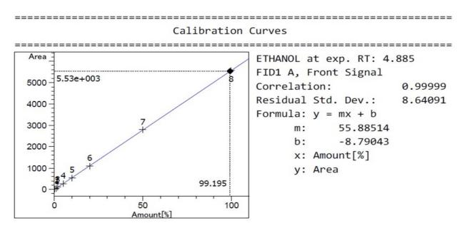
Figure 1. Calibration curve of ethanol standards.
