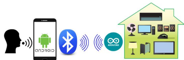
Figure 2: System Architecture of Smart Home Automation System
