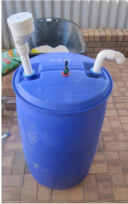
Figure 6a: External view of the digester
