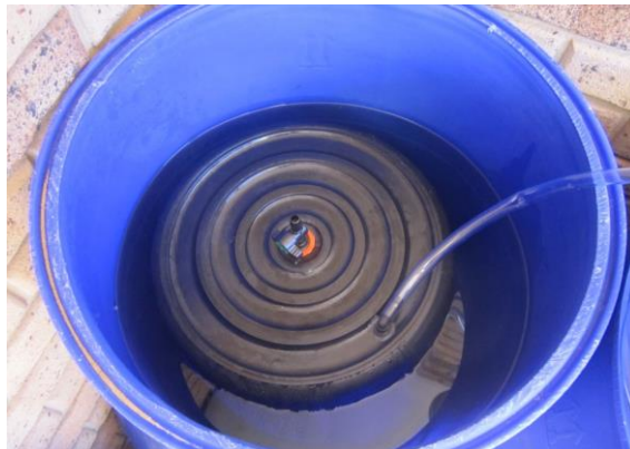
Figure 7: The collector is an inverted garbage bin submerged in water
