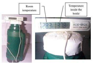
Figure 1: Device used for maintenance of temperature until dispatch to laboratory
