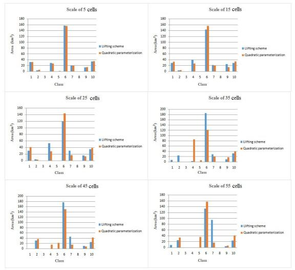
Figure 7: Comparison of landforms extracted using the two methods (Case 2). 1: Canyons, deeply incised streams, 2: Midslope drainages, shallow valleys, 3: upland drainages, headwaters, 4: U-shaped valleys, 5: Plains small, 6: Open slopes, 7: Upper slopes, mesas, 8: Local ridges/hills in valleys, 9: Midslope ridges, small hills in plains, 10: Mountain tops, high ridges.
