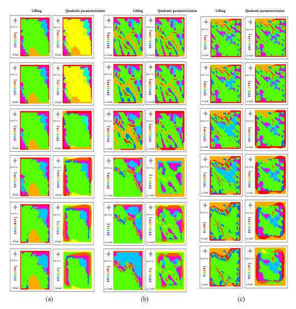
Figure 5: Landform classification for the multiscale DEMs for: (a) Case 1 (b) Case 2 (c): Case 3. 1: Canyons, deeply incised streams, 2: Midslope drainages, shallow valleys, 3: upland drainages, headwaters, 4: U-shaped valleys, 5: Plains small, 6: Open slopes, 7: Upper slopes, mesas, 8: Local ridges/hills in valleys, 9: Midslope ridges, small hills in plains, 10: Mountain tops, high ridges
