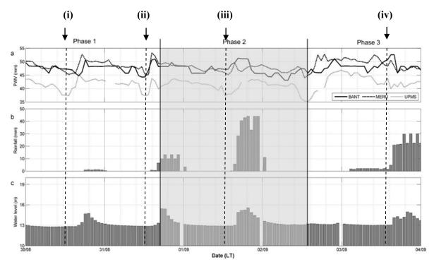
Figure 2: Variation of (a) PWV at the three GPS stations, (b) rainfall and (c) river water level for the five day period from 30 August to 4 September 2013, where the flash flood event occurred on 1 September.
