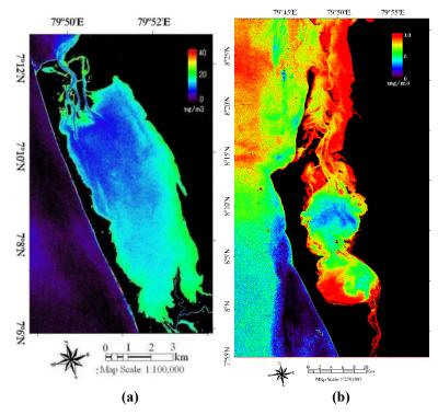
Figure 4: Chl-a distribution maps derived using the ASTER/OC3 based method: (a) Negombo estuary on Feb 16, 2009. (b) Puttalam lagoon on Jan 31, 2009.
