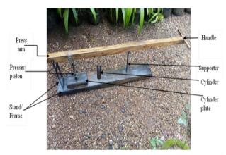
Fig 4. Homemade briquette machine
