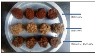
Fig 5. Briquettes used by primary material
