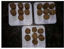
Fig 7. Briquettes used by primary and wastepaper material
