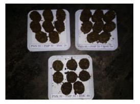
Fig 8. Briquettes used by primary and cow dung material
