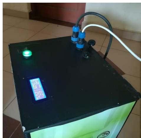
Fig. 7. The LCD display and indicator connection after installation
