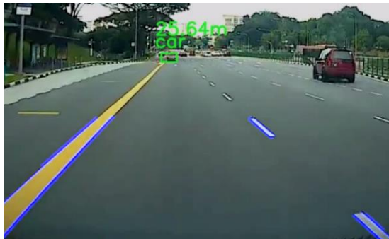
Fig. 4. Detected lanes in a road
