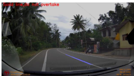
Fig. 10. Solid line detection
